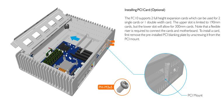
Fit the expansion card to case by carefully aligning it with the opening and ensuring the lower side of the card bracket fits into the lower support. Once the cards are in place, secure them to the PCI mount using the screws provided.
