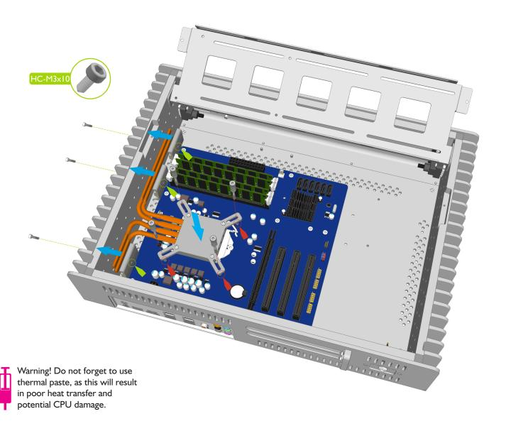
Carefully lower the heatpipe/CPU mount assembly into the case and place it onto the CPU, ensuring the heatpipes only make contact with the heatsink once the assembly is resting centrally on the CPU. Fit the 4 spring loaded screws to the motherboard (into the CPU mounting nuts), but do not fully tighten yet.
