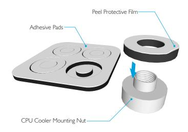
With the motherboard turned upside down, located the CPU cooler mounting holes. The hole position will vary depending on the brand and model of CPU. Peel the protective film from the adhesive pads and stick the nuts to the underside of the motherboard ensuring they correctly align with the holes. The slightly raised rim of the nut should fit through the motherboard CPU mounting holes.
