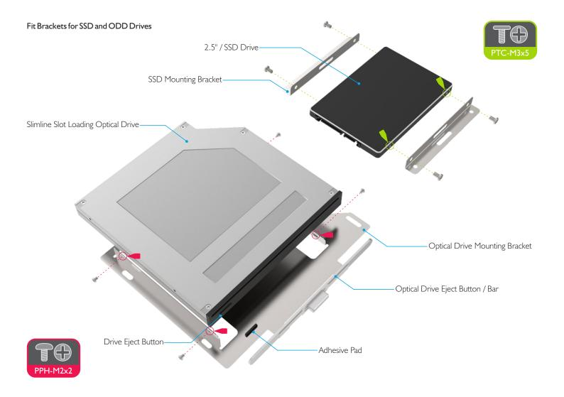
SSD and ODD drives that fit to the upper side of the tray require brackets to be attached first. If you purchased the OPTICAL version of the FC8, it will include an optical drive mounting bracket, otherwise the kit will include and extra set of 2.5" mounting brackets (2 for each drive).
