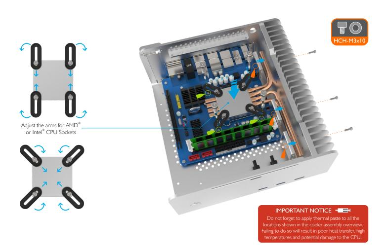
Secure the heat pipes to the heat sink using the 3 heat sink mounts as hex screws that pass from the outside of the case (between the fins). There are a number of holes along the heat sink to allow for different heat pipes and CPU locations, so ensure you select the appropriate location to evenly apply pressure on the heat pipes. Before fully tightening the heat sink mount screws, ensure once again the CPU mount is centrally located over the CPU.
