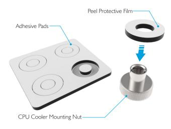
With the motherboard turned upside down, located the CPU cooler mounting holes. The hole position will vary depending on the brand and model of CPU. Peel the protective film from the adhesive pads and stick the nuts to the underside of the motherboard ensuring they correctly align with the holes. The slightly raised rim of the nut should fit through the motherboard and protrude slightly from the top side of the PCB.
